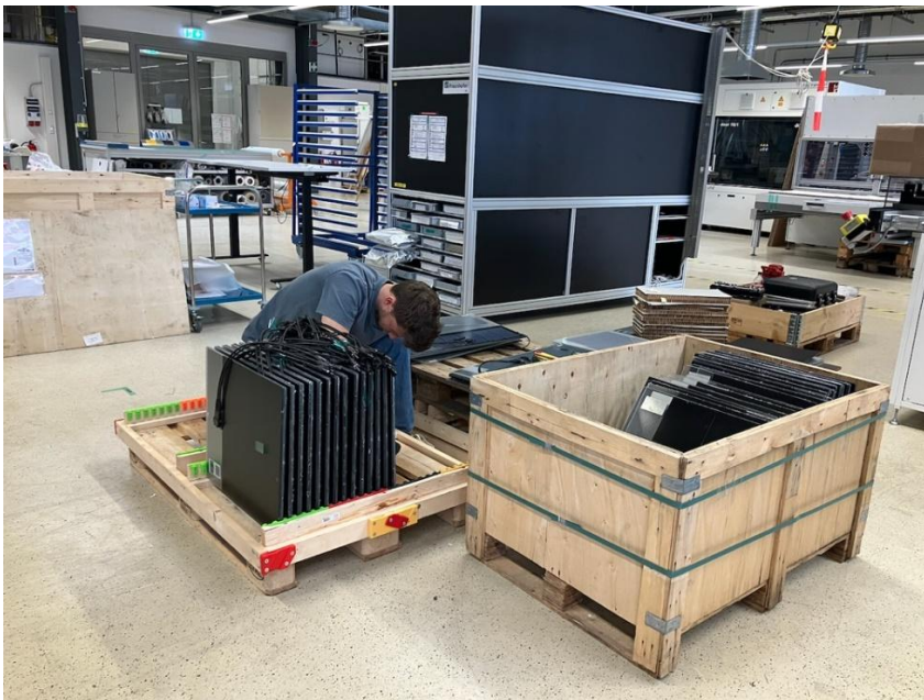
2. New 3D Printed Reusable Packing case versus old single use wooden case.
