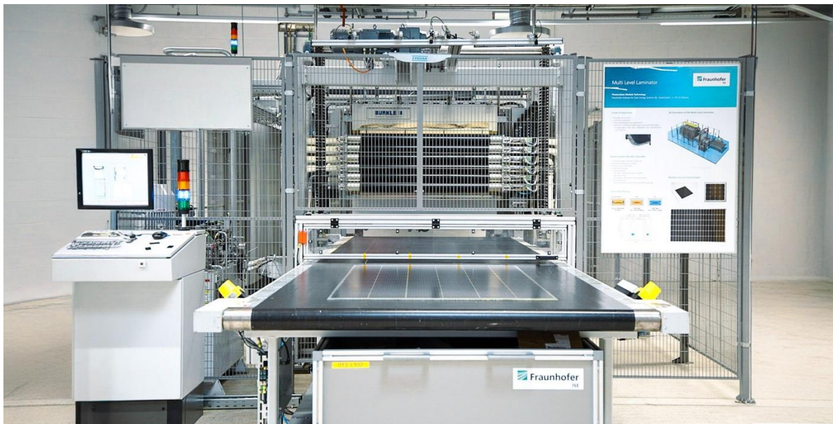
Figure 17: Photovoltaic module laminator capable of performing plate-membrane, plate-plate laminations as well as cooling arranged in stacks.
